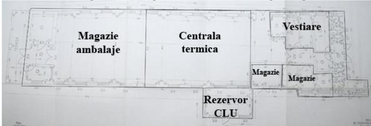
The building is made of brick, with concrete foundation, concrete flat roof with tar paper covers, with a built area of **482mp**, is made up of packaging warehouse, central heating, reception office, two toilets, two warehouses, and 2 changing rooms with a usable area of **386 sqm**.
